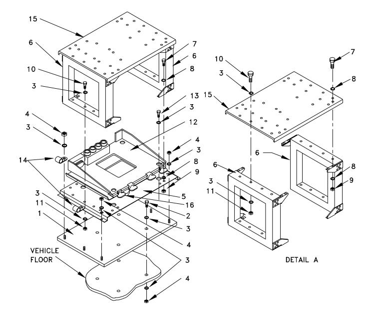
5.2 Installation of Mounting Base, Electrical Equipment MT-6352/VRC (mounting base). Continued.
