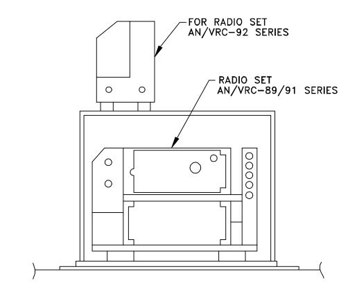
Figure 5-1(2). MK and Radio Installation: Radio Equipment Locations
