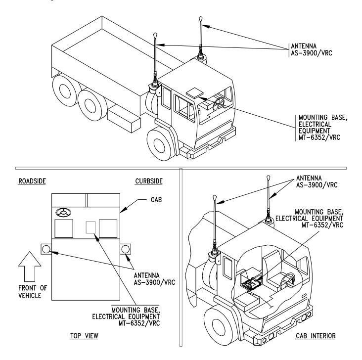
Figure 5-1(1). MK and Radio Installation: MK Equipment Locations
